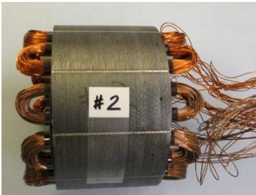
Figure IV-56: Stator constructed with the HT film developed on this project as slot liner.
