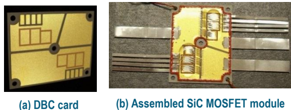
Figure III-62: DBC design and SiC switch phase-leg modules fabricated using the DBC cards.
