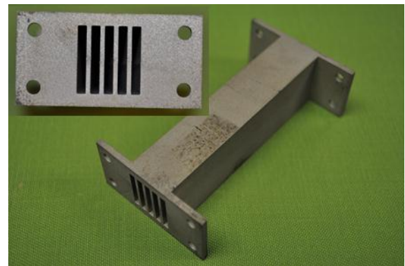
Figure V-33: Baseline aluminum fin block sub-module test section.
