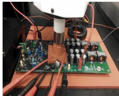
Figure II-31: Experimental setup for dynamic characterization of a 600 V, 5 A GaN FET.
