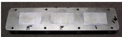
Figure III-151: Substrate to Coolant Manifold Attachment.
