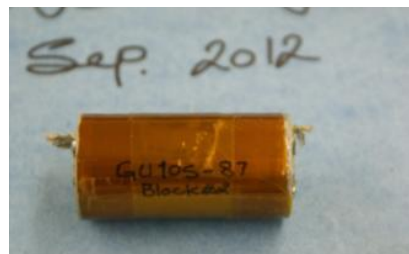
Figure III-155: Blisters on shorted cap.
