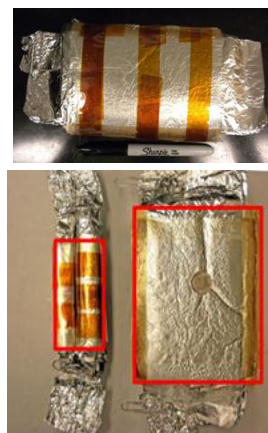
Figure III-133: Stacked capacitor (top) Stacked vs. rolled.
