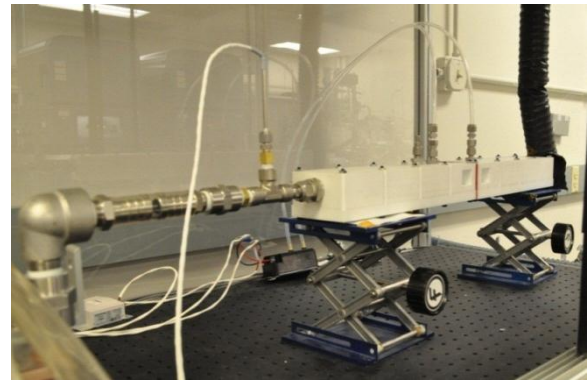
Figure V-32: Test section for testing baseline aluminum fins with two heaters for model validation; pressure calibration testing shown. (Photo Credit: Scot Wayne, NREL).
